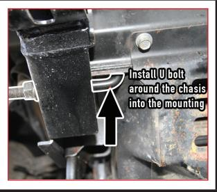
• The U bolt should hold the mounting bracket as shown.
