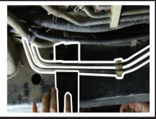
• Insert The larger bolt in the top hole then tighten slightly with nut provided.
