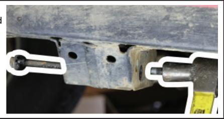
• There is 2 capture bolts in the fitting kit insert 1 in the round hole in the chassis.
