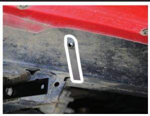
• On the passenger side of the vehicle there is a wiring harness on the inner side of the chassis with a screw driver lever it out of the way
