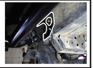
• Slide the plate behind the brake line and wiring harness on the centre bracket.
