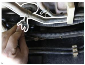
• Using the smaller bolt insert it through the bottom hole of the plate( Plate Has thread).
