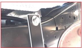
• Align step to the maximum forward position and maximum height position. Tighten all bolts evenly.
