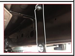
• Attach rear bracket. Ensure that all top bolts are located UNDERNEATH all wiring and brake lines during installation.
