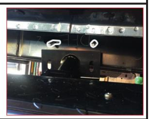
Support step to allow for lifting and levelling.
