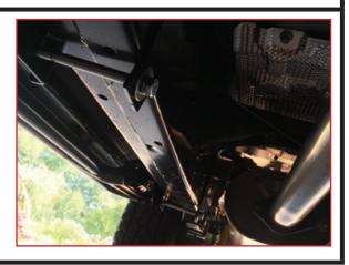
• Install passenger side step as per drivers side order. The rear bracket installation requires temporary removal of fuel tank underbody protection (4 x nuts for removal) and permanent removal of 1 x brake line bracket bolt which is subsequently supported by the rearmost bracket.
