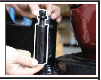
• Once the arm is on, it will lock straight in; the locking bracket can also be adjusted.
