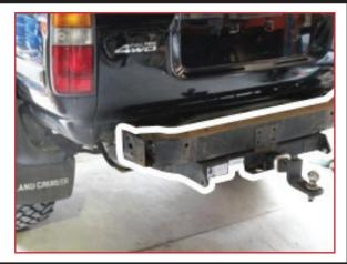
• Place the bar on the vehicle – this will be made easier if two people assist each other in order to guide the bar safely on to the chassis.
