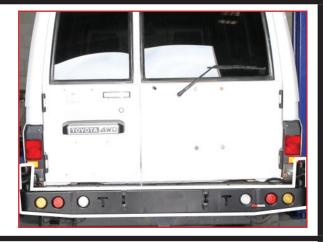
• THERE IS 3 BOLTS AND NUTS ON THE REAR OF THE BAR AND 4 BOLTS ON THE SIDE OF THE CHASSIS (ONLY SEMI TIGHTEN)
