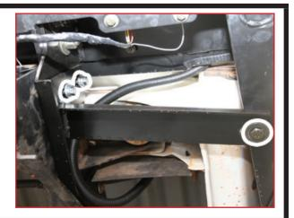
• Remove the checker plate there is 4, 19mm bolts that dolt to the centre of the chassis
