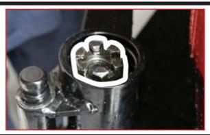
• The cap secures the nut in place
