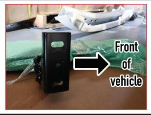
• Unbolt the bracket holding the fuel line, move it so that it is not in the way for fitting.
