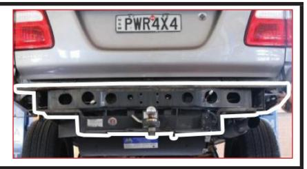
• Fitting the bar does not require you to remove the Tow Bar, however on some vehicles you may be required to unbolt the side mounts of the tow bar which connect to the chassis.
